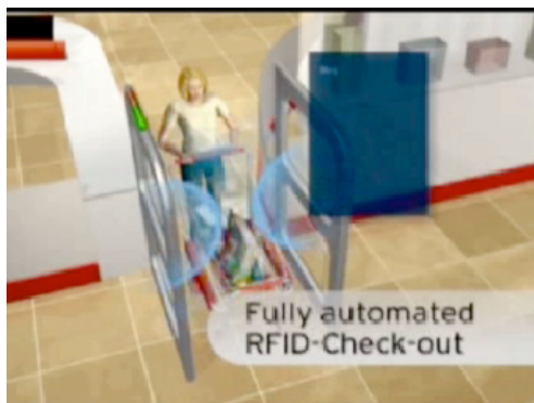
Figure 9: Automatic check-out of products tagged with RFID chips (Metro Group in 2004)
